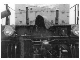
**Case # 2 -** The plaintiff suffered fatal injuries when he fell between moving cars while riding a cut due to the bent platform shown to the right. The railroad's post accident inspection report included the following entries: "no defect found . . ." and "safety appliance on this is in proper limits and secured." Unfortunately for
